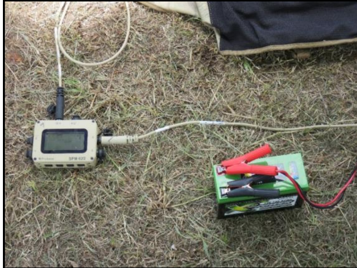
Figure 40. Charging the Roving Blue WPS with Filtration Battery with the Squad Power Manager with 100W Solar Blanket
