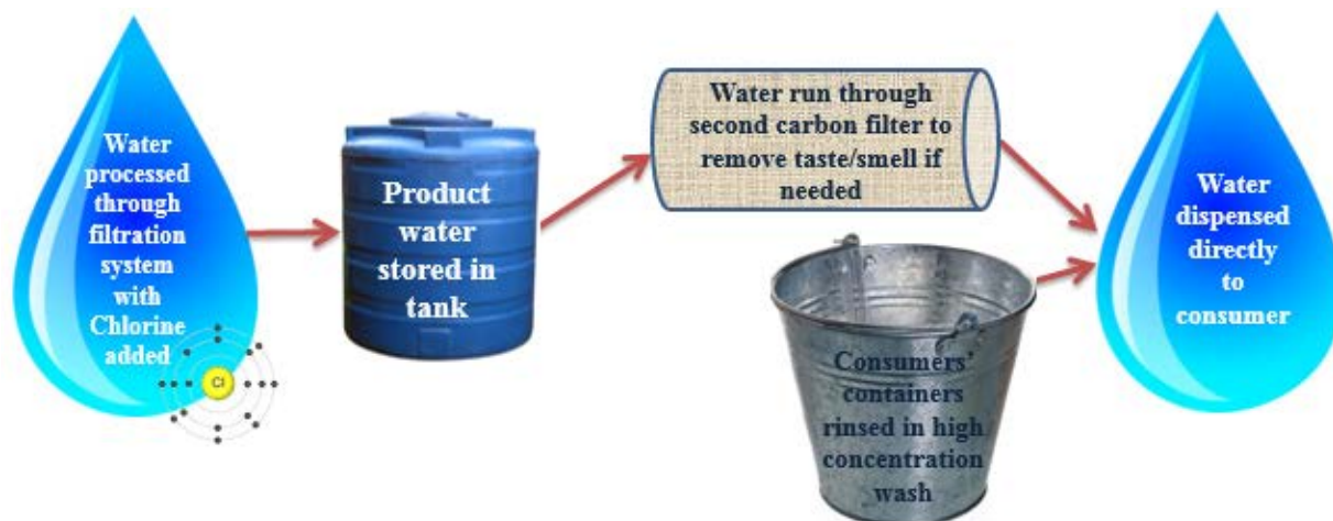
Figure 1. Product Water Distribution Path 1
