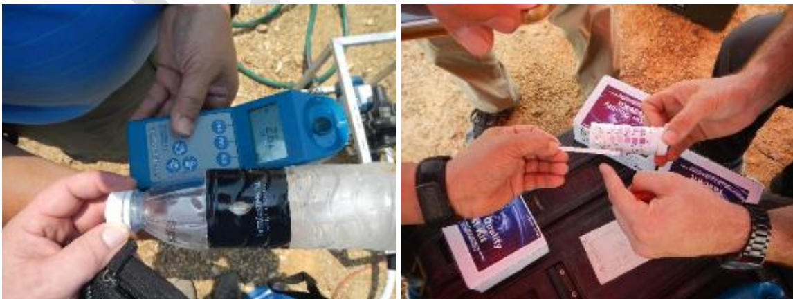
Figure 12: TDS Testing (Left) and Chlorine Test (Right)
