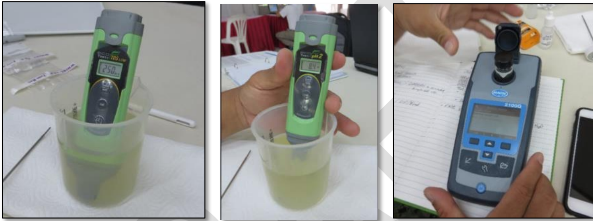
Figure 32. Oakton EcoTestr TDS Low Pocket TDS Tester (left) Oakton EcoTestr 2 Pocket pH Tester (center) Hach 2100Q Handheld Turbidity Meter (right)
