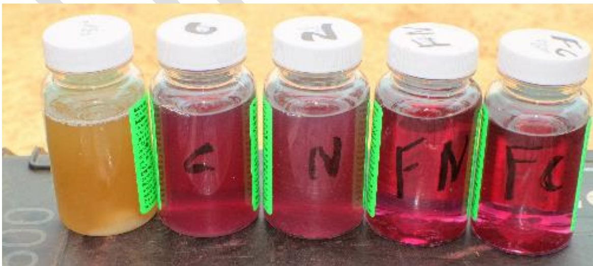
Figure 14: Bacteria Testing (from left to right, source, chlorine, SilverDYNE, Filtered w/SilverDYNE, and Filtered w/chlorine)
