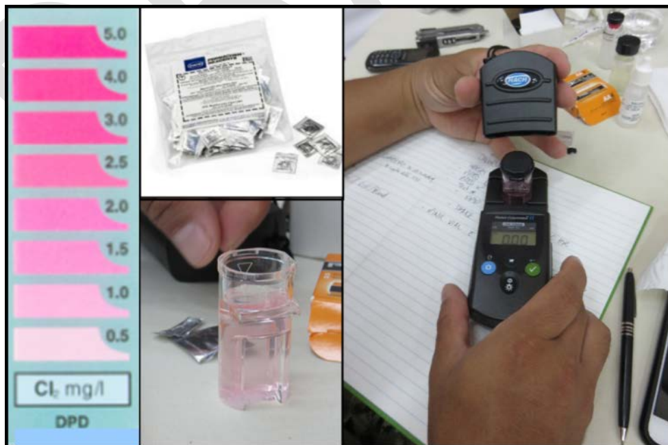
Figure 33. DPD Reagent, Scale, and Hach Chlorine Pocket Colorimeter II
