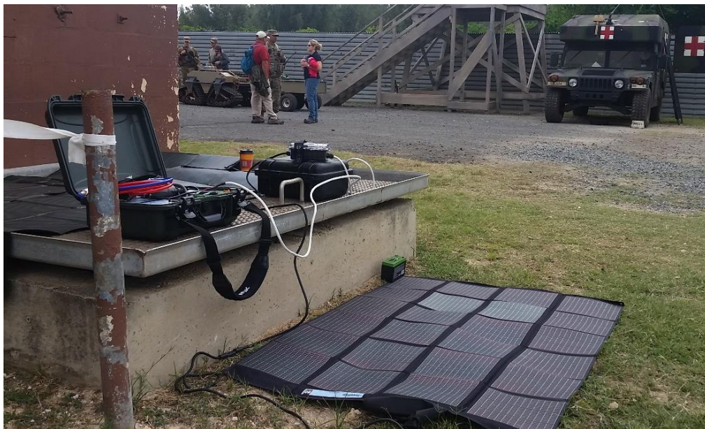
Charging the batteries prior to deployment. Shown is the Roving Blue MVP-M w/optional 65 Watt Solar Panel, The Solar Panel was specifically developed for Roving Blue's technology by Solar Stik™, Inc. , Saint Augustine, FL.
