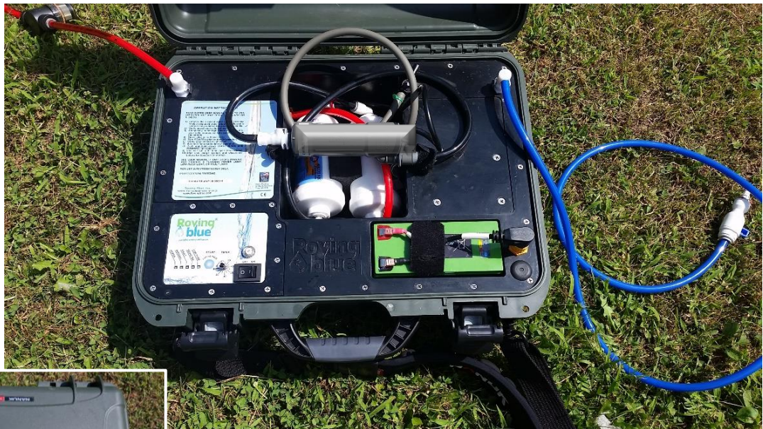
-Everyone liked the fact that the entire system comes in an all-in-one small ruggedized case that weighs less than a single case of water (23 lbs), and can consistently produces about a liter of water a minute. (30 gallons in 2 hours)
